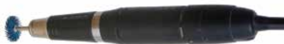
Micromotor handpiece with blue 400-grit abrasive 3M Bristledisc™ in the collet. Tool length is 6½" (17cm)
