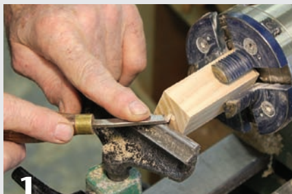
1 Make a centered starter hole using the long point of a skew.
