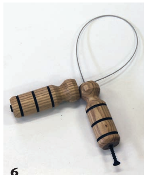
6 Affix the wire to the handles using drywall screws. The wire is inserted through the top all the way to the bottom of the handle, where the drywall screw pinches it firmly in place. Note the screw at right is left unfastened for the purpose of illustrating the tool's construction. Tighten both screws to hold the wire firmly in place prior to using the tool.
