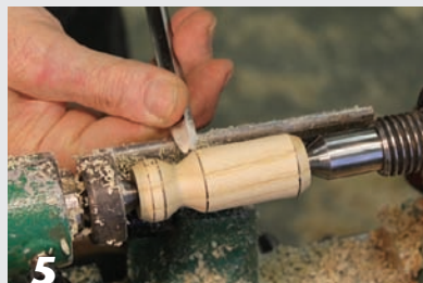
4 With the blank mounted between centers, turn it round and add details. A cove near the top aids in gripping the burning wire during use.
